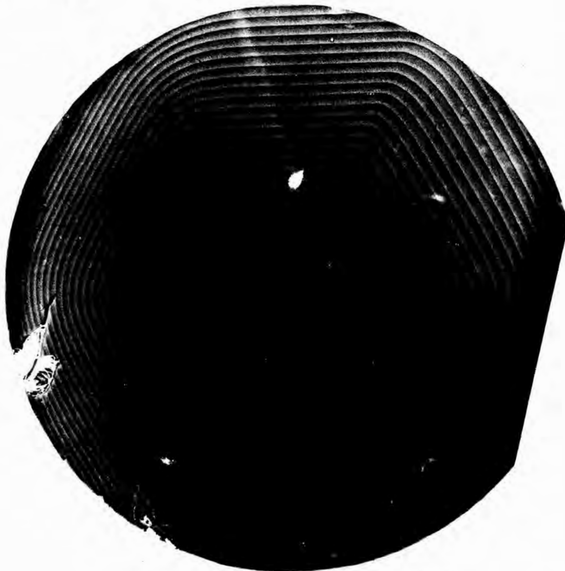
A growth spiral on the surface of silicon carbide crystal
